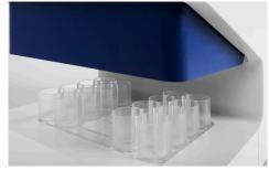
The plastic micro-injection-molded consumable allows 4 samples to be prepared simultaneously (see picture). Source: z-werkzeuabau-ambh
